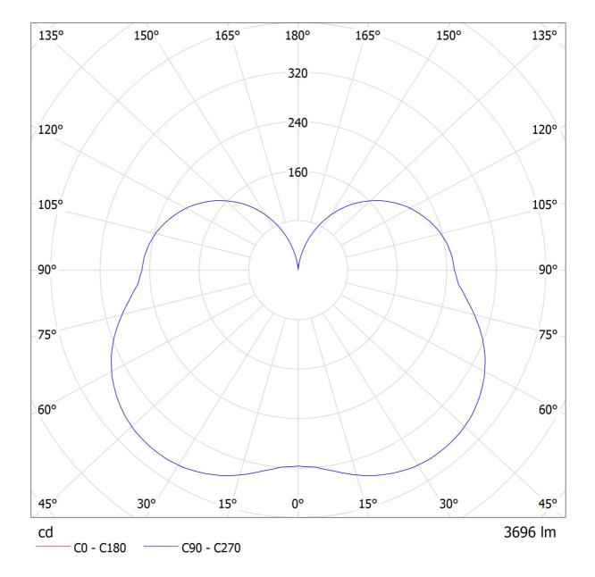
Luminaire: Lucis IC.K1.440.X IZAR C LED Lamps: 1 x LED 252/160-G5
