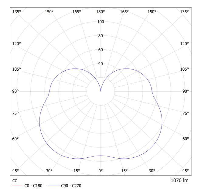
Luminaire: Lucis IC.K2.150.X IZAR C LED Lamps: 1 x LED 103/73-G5
