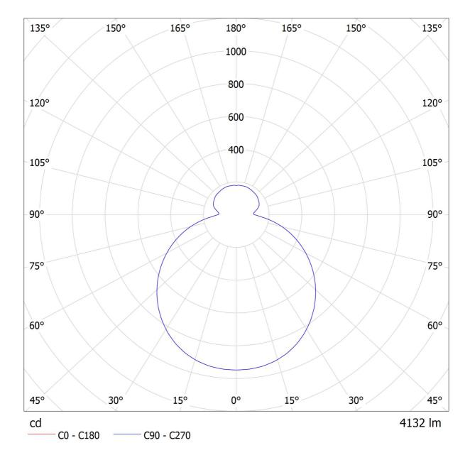
Luminaire: Lucis PS13.K4.Z600 ZERO LED Lamps: 1 x LED G5
