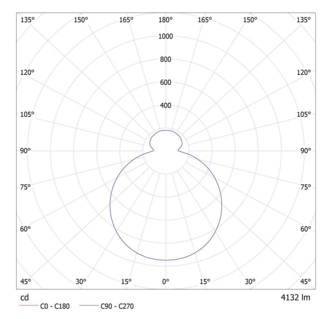
Luminaire: Lucis S46.K4.Z600 ZERO LED Lamps: 1 x LED G5
