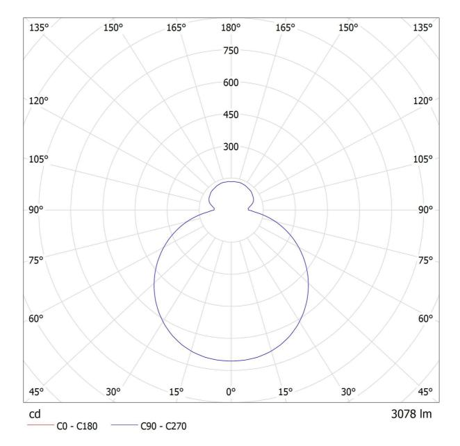
Luminaire: Lucis S43.K3.Z500 ZERO LED Lamps: 1 x LED G5
