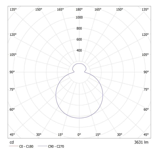
Luminaire: Lucis S34.K2.Z415 ZERO LED Lamps: 1 x LED G5
