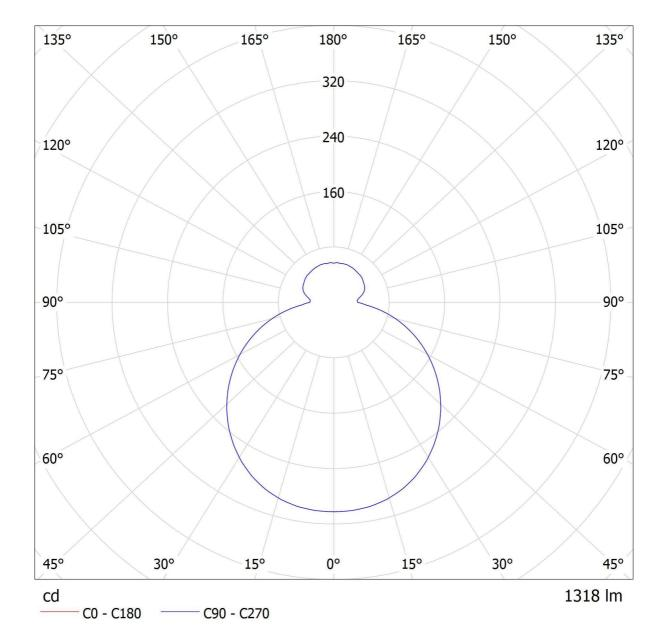
Luminaire: Lucis S24.K1.Z280 ZERO LED Lamps: 1 x LED G5
