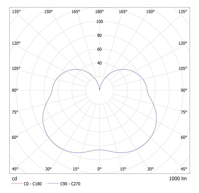
Luminaire: Lucis ZL1.IC.L1.150.X IZAR C LED Lamps: 1 x LED 2908
